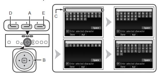
1. When the on-screen keyboard shown above is displayed, touch the center FUNCTION button (A) to switch to a keyboard having the characters you want to use.
